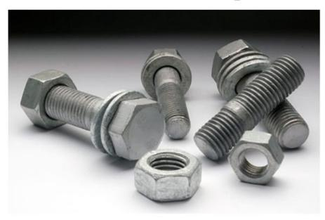
Hot-dip galvanizing (HDG) is a process that coats steel nuts and bolts with zinc to protect them from corrosion. The zinc coating is durable and low maintenance, and can last for 50–70 years in most environments.
